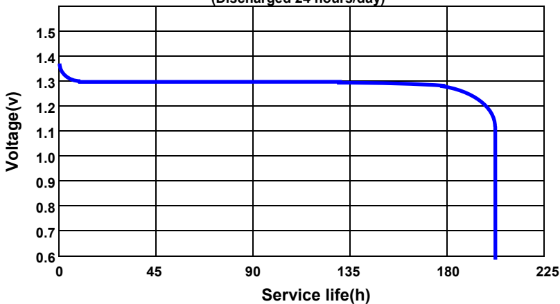
DISCHARGE CHARACTERISTICS AT 1500Ω 25°C 60%RH (Discharged 24 hours/day)
